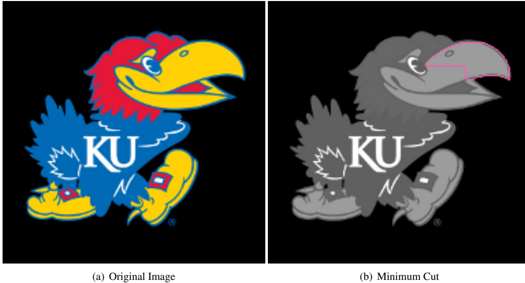
Figure 2. A sample result. The source was placed on the Jayhawk’s beak, and the sink in the upper left corner. The pink border represents the minimum cut.
